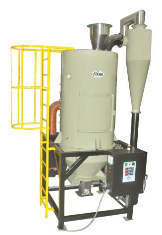
A Nu-Vu Conair crystallizing system will allow you to convert amorphous PET (granules / flakes) to a crystalline state that can be dried. The drying can occur at an elevated temperature to obtain low moisture levels without the fear of agglomeration.
